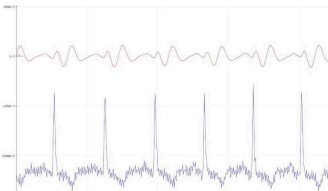
Fig.5. Representation on the Arduino serial monitor. The unfiltered real electrocardiogram signal is shown in blue, while the signal passing through the 8-13 Hz filter is shown in red.
